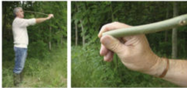
Figure 10. Measuring a tree by the use of a stick to measure tree height
